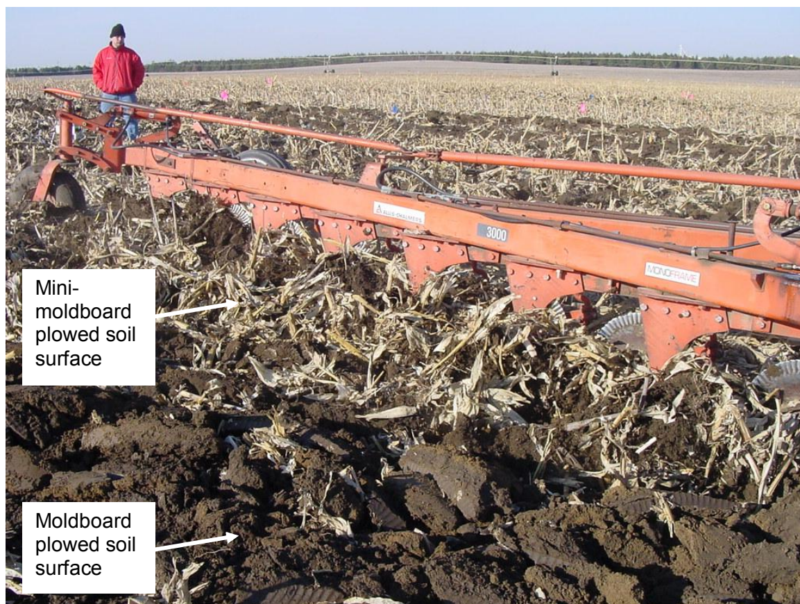
Figure 1.3. The mini-moldboard plow (miniMP) in operation adjacent to a plot tilled with a regular moldboard plow (MP). Note the difference in residue cover and soil roughness with the two implements.
