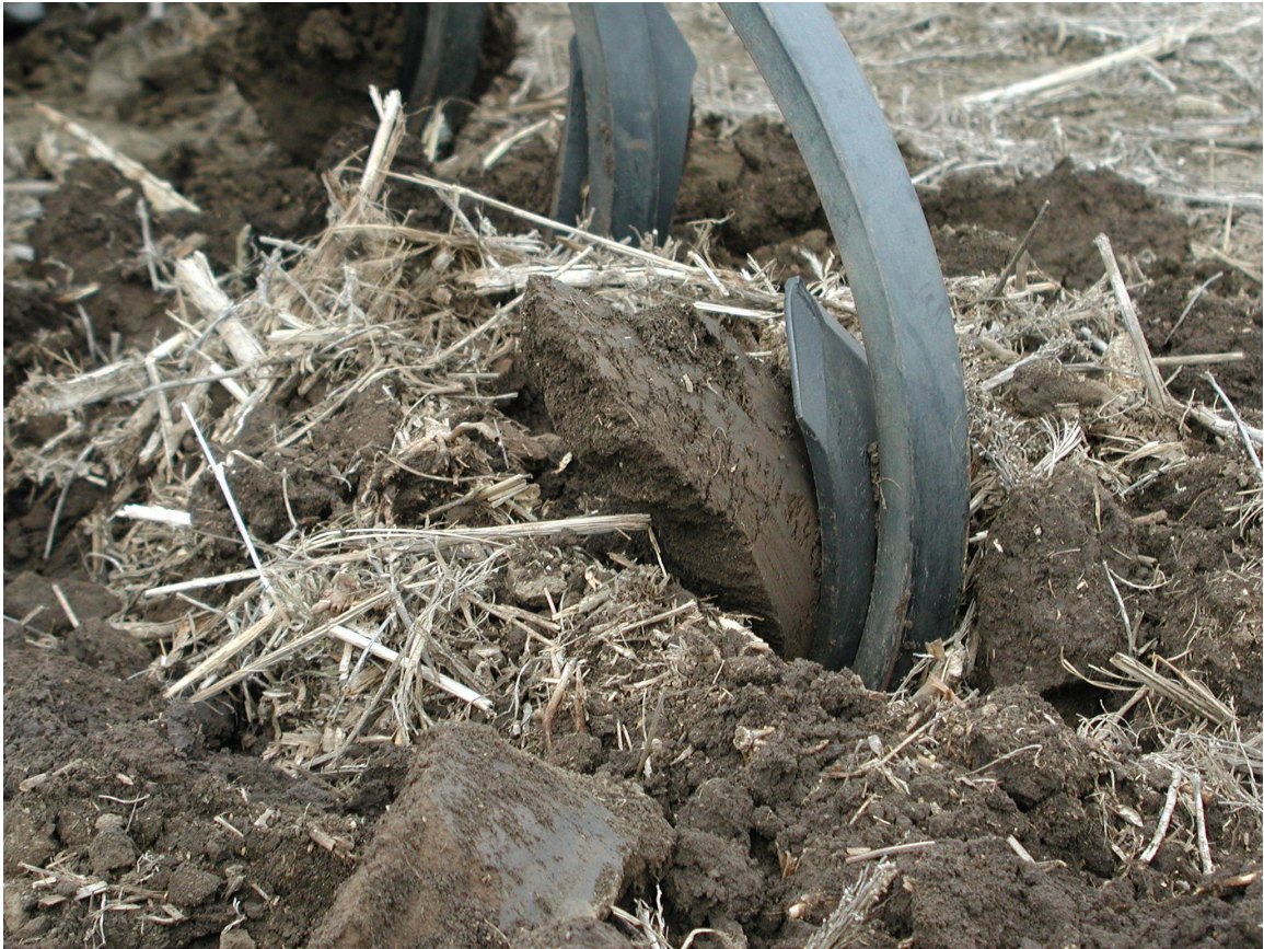
Figure 1.2. The chisel plow to 20-cm and 30-cm (Ch20 and Ch30) used in this study was equipped with 10-cm-wide twisted shanks that bring some deep soil to the surface.
